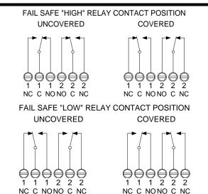
**FailSafe High** means that the relay will energize when the paddle is uncovered and will de-energize when the paddle is covered. In this mode, a failure will cause the relay contacts to indicate that the paddle is covered, whether it is or not.
